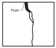
Figure 5. Crack Sealing
