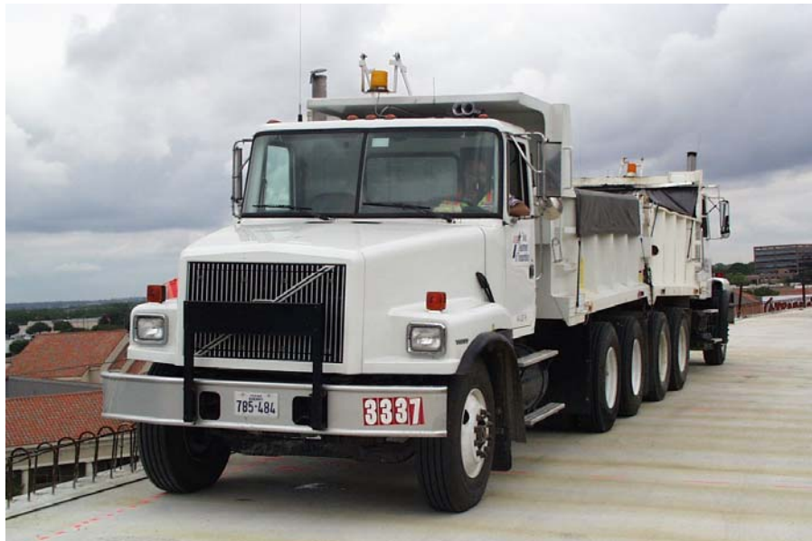
Figure 6.20 Truck Positioning During K Live Load Test
