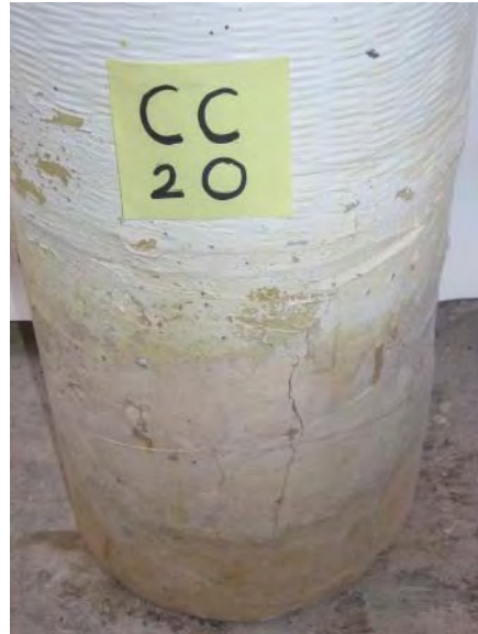
Crack over rebar A in unwrapped region.
