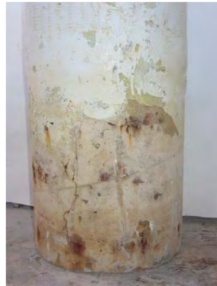
Crack and rust stains over rebar A.
