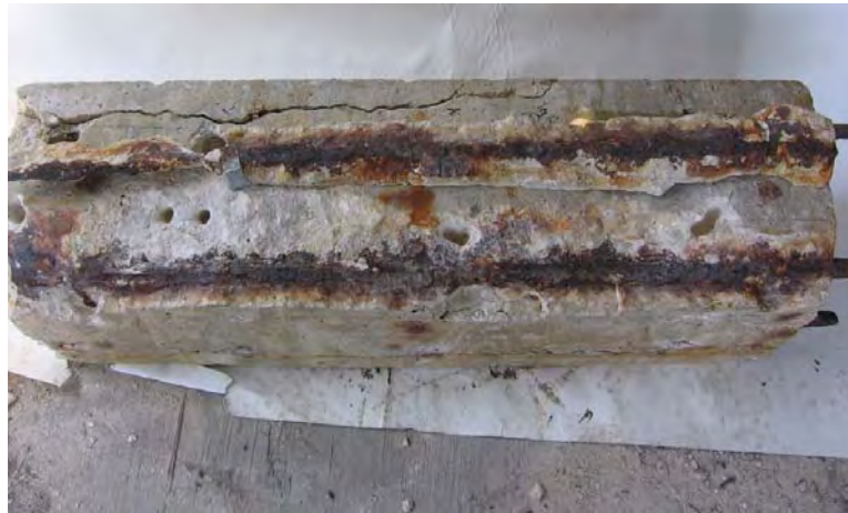
Figure 3.8 Corrosion of bars in unwrapped specimen
