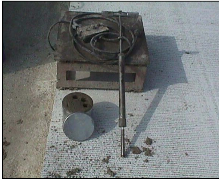
Figure 4-4: Vibration table and Pentrometer used on site
