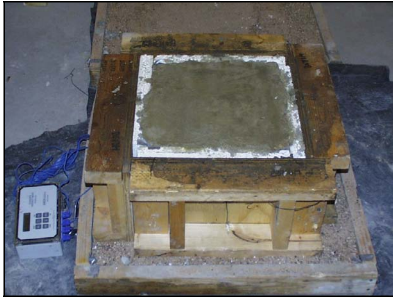
Figure 4-41: Small insulated concrete specimen in the environmental chamber
