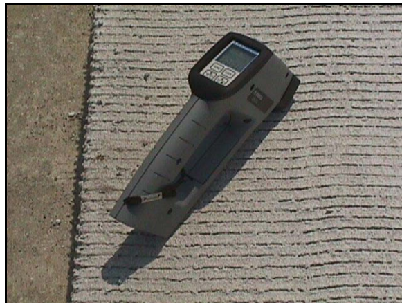
Figure 4-3: Handheld infrared thermometer used during the field work
