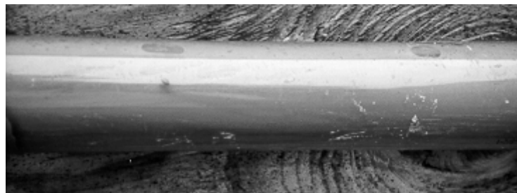
Figure 3.5 TxDOT Grout – Bubbles Traveling Toward Intermediate Crest 34
