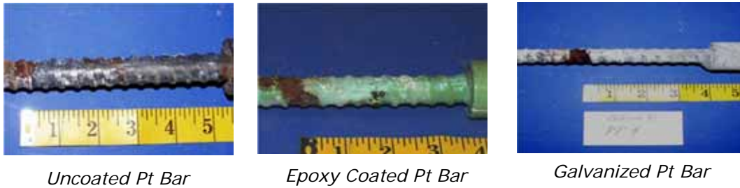
Figure 3.26 Bar Coating Performance when Subjected to Localized Attack 37
