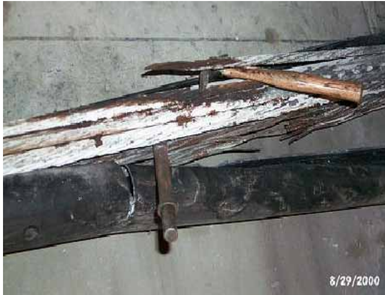
Figure 2.8 Failure of Tendon 28-6 on the Mid-Bay Bridge 16
