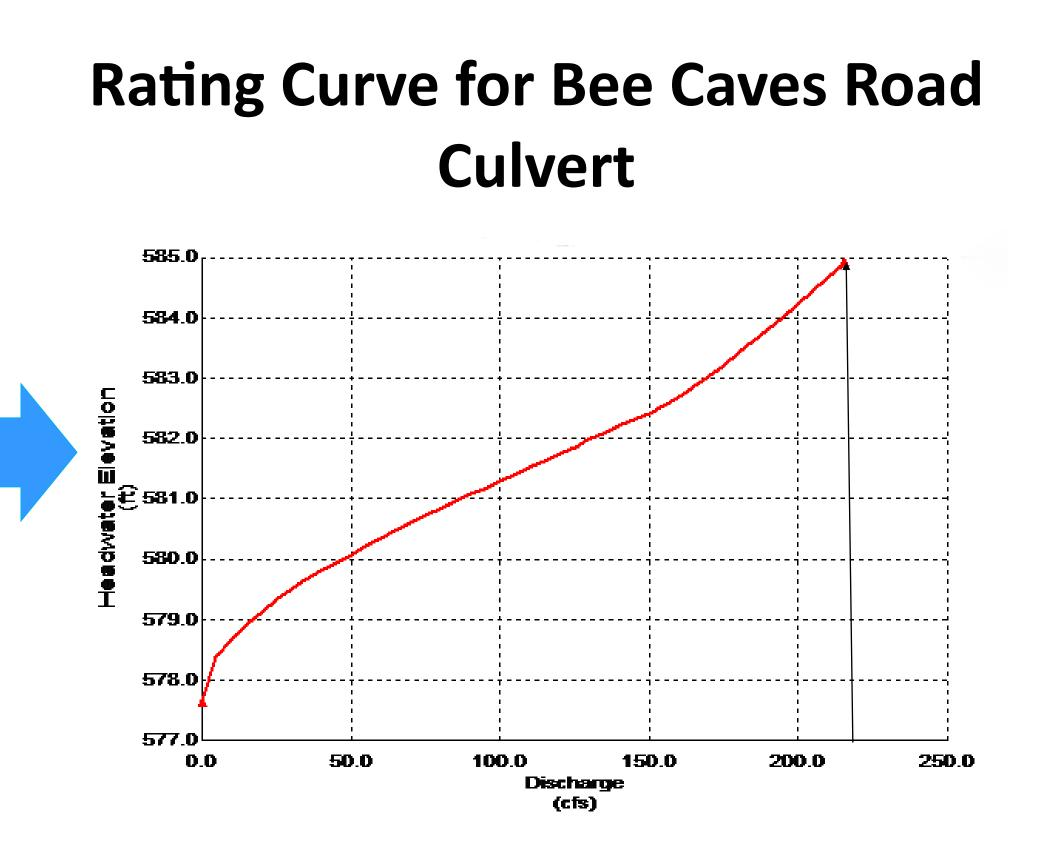
**Connecting forecasted streamflow and culvert rating curves to** predict flooding at these locations up to 15 hours in advance!
