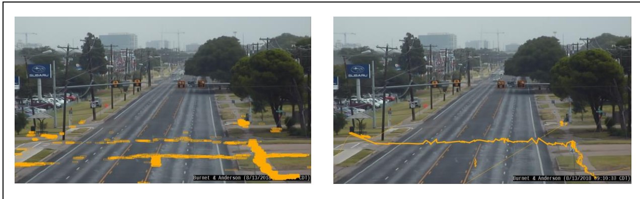
Figure 10. Hotspot view of pedestrian detection location (left); (right) inferred pedestrian crossing event based on tracking algorithm. The missed crossing event in the pedestrian crossing summary (right) is due to significant speed differences (pedestrian running in missing track).
