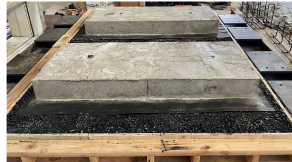
CSB + 1 in. HMA layer with bond breakers
