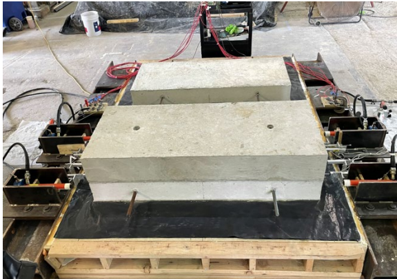
CSB with bond breakers
