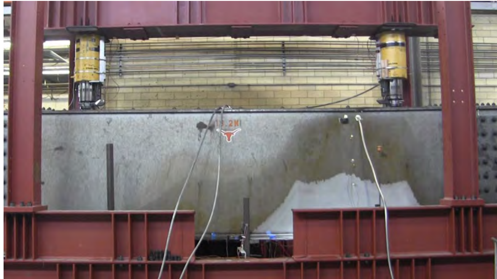
Post-Fracture Loading using 10,000 psi pneumatic pump
