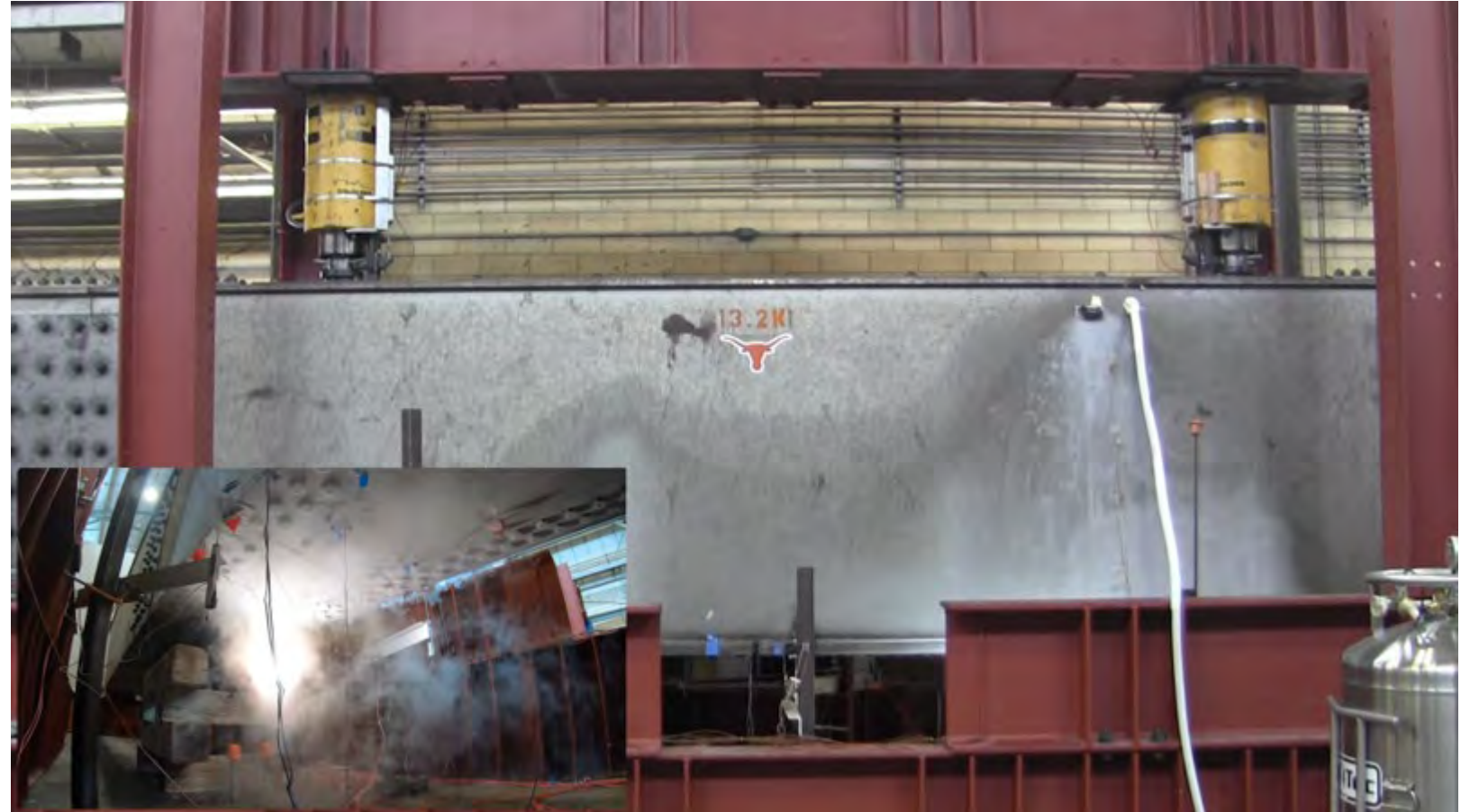
Fracture Loading using 3,000 psi HPU
