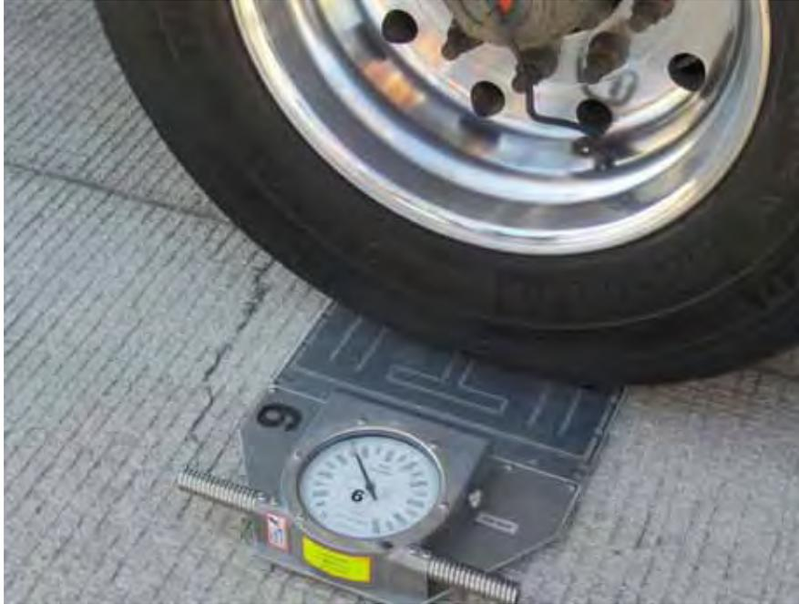
*Figure 5.11: Weighing one of the truck axles*
