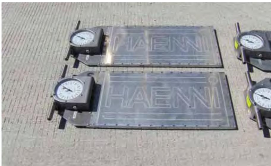
*Figure 5.10: TxDOT's portable scales*
