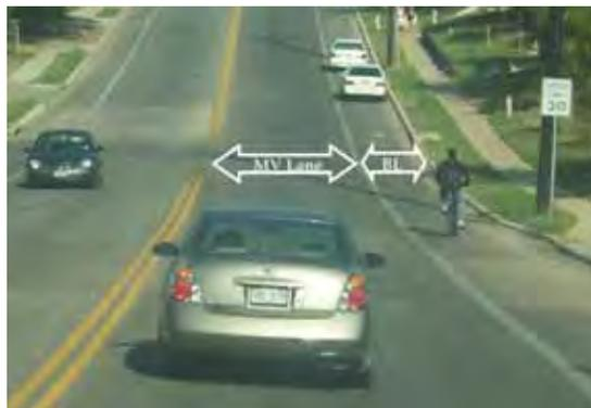
*Figure 3.8: Example of motor vehicles parking in the bicycle lane*
