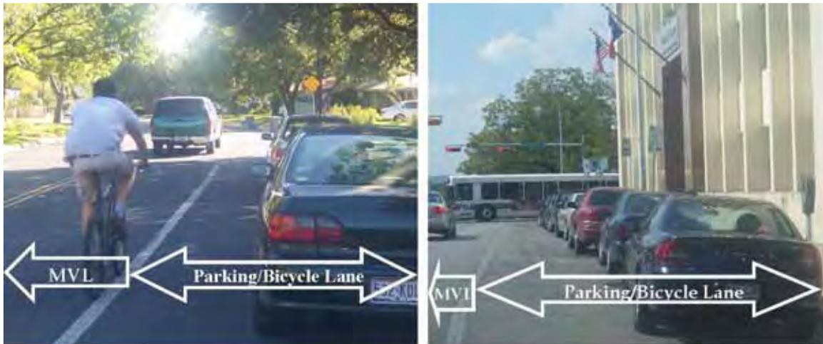
*Figure 3.9: Examples of combined parking and bicycle lane*
