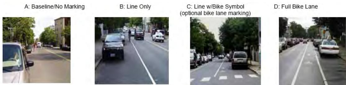
*Figure 2.7: Added Components of Bicycle Lane*
