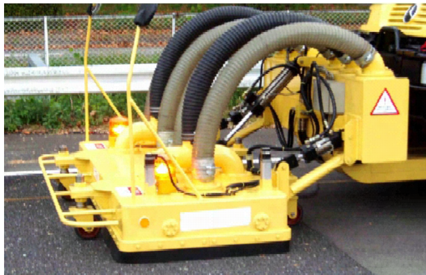
Figure 5 - Cleaning machine with high-pressure air only from PWRI (2005)
