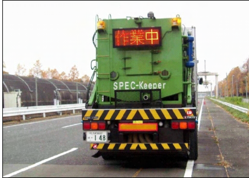
Figure 4 - The Spec-Keeper cleaning machine in Japan from PWRI (2005)
