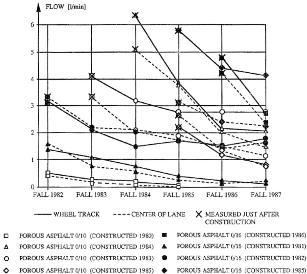
Figure 1 - Drainage potential over time (Isenring et al., 1990)
