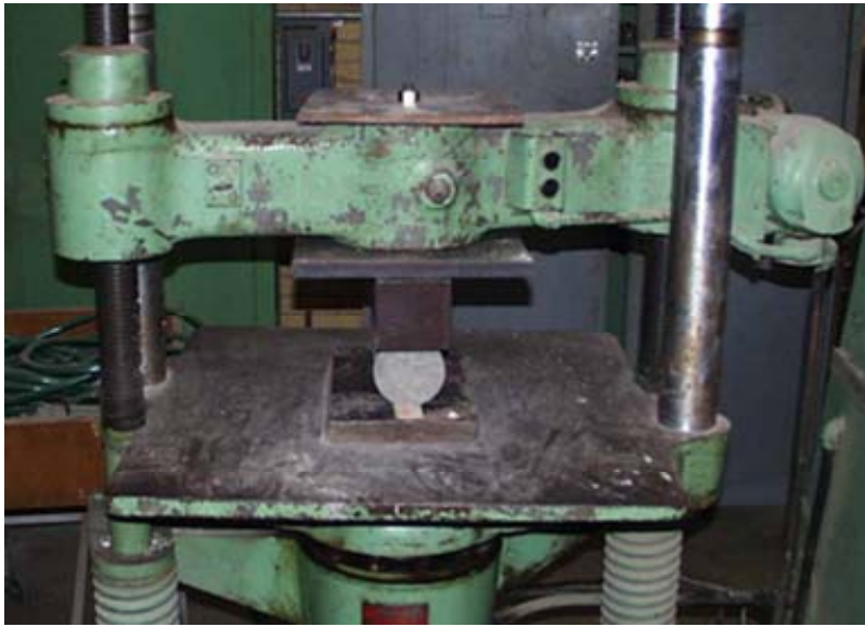
Figure 3-7 ASTM C496 Standard test method for determining the splitting tensile strength of concrete.
