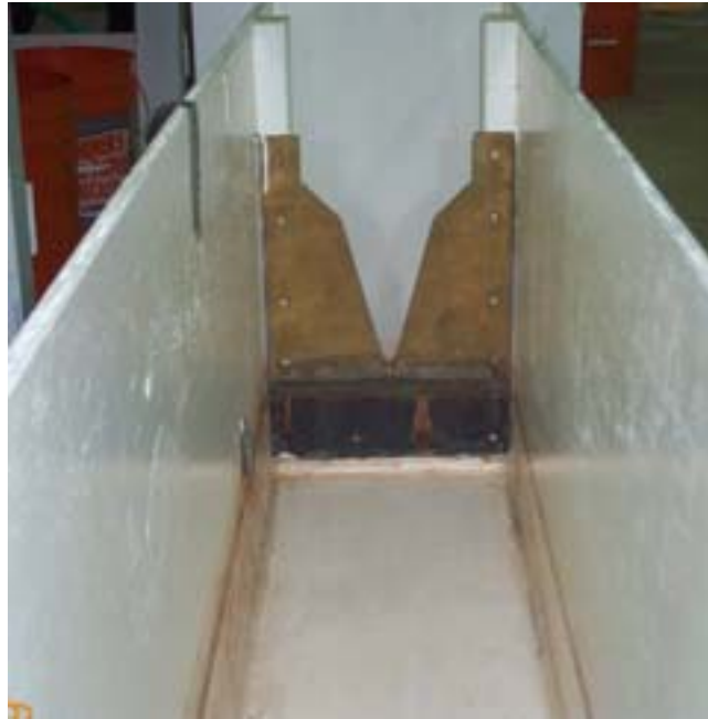
Figure 12. Flow measurement channel.
