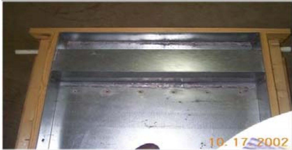
Figure 11. Effluent launder assembly.
