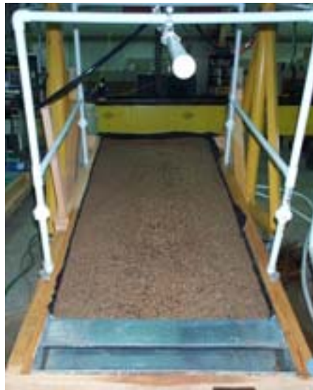
Figure 14. PVC support structure for header pipe.
