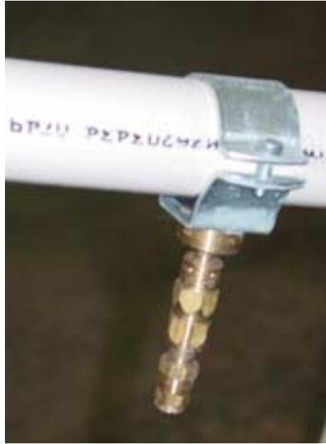
Figure 13. Erosion control study nozzle assembly.
